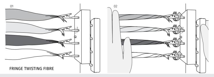
Clamp fringe twister to a table. Divide fibre/sliver into even desired thicknesses. Clip each length in place.
