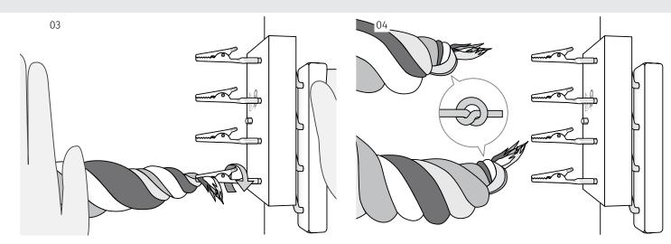
Holding onto the ends, unclip and place all 4 opposite ends into one clip and rotate anti-clockwise.
