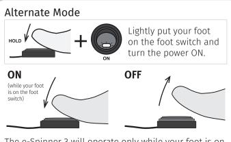
The e-Spinner 3 will operate only while your foot is on the foot switch. Lift your foot off and the e-Spinner 3 will stop. **NOTE:** Ensure the e-Spinner 3 is switched OFF before removing the foot switch plug.
