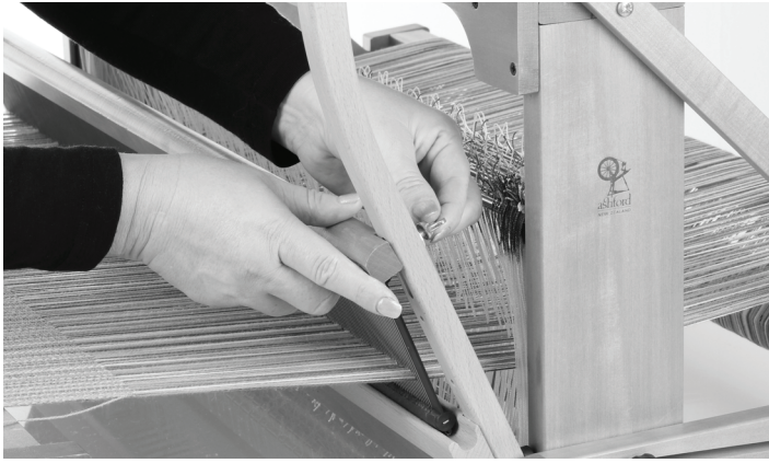
10. Locate the top beater rail back into position and secure with bolts, washers and wing nuts.
