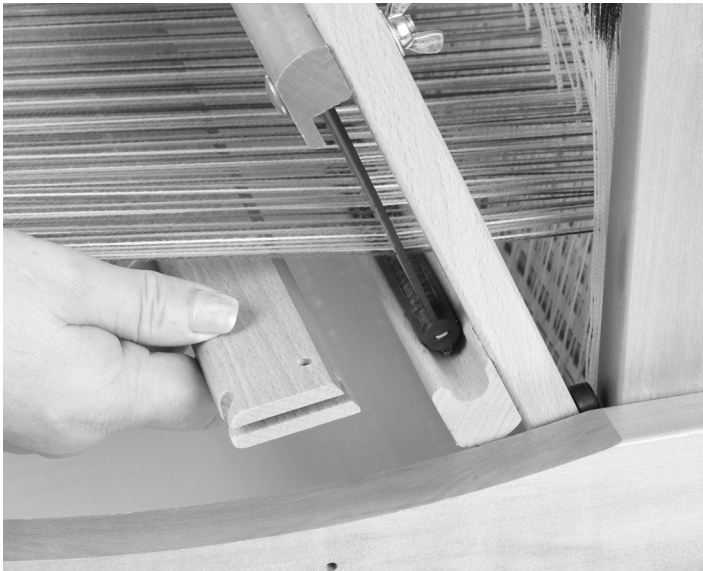
12. Position the Shuttle Race under the warp with the tapered edge facing the reed.
